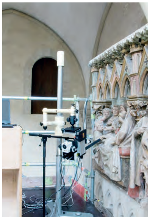
Fig. 10 (right) Measuring head of the mobile Raman microspectrometer in use at the relief of Naumburg west rood screen (Photo Jacqueline Menzel)
