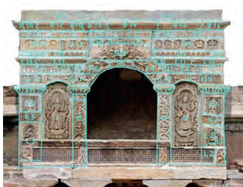
Fig. 6 (left) Patan, Bhandarkhal Tank Pavilion, graphic documentation of the blocks, their relative positions in the structure and the joint net, (Institute of Conservation, University of Applied Arts Vienna, 2010)
