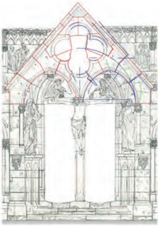
Fig. 13 (left) West rood screen of Naumburg Cathedral, east side, central gable (drawing) with drawn in sketches and joints. Red: jointing arrangement, blue: projected engraved drawings from the west choir, green: engraved drawings on the gable. (Author: Ilona Dudzinski)
