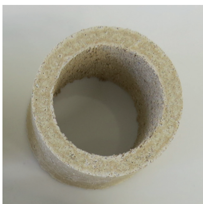
Pic. 2 and 3 Cylinders glued together with the mixture of NHL5 and water. Photos: Varje Õunapuu
