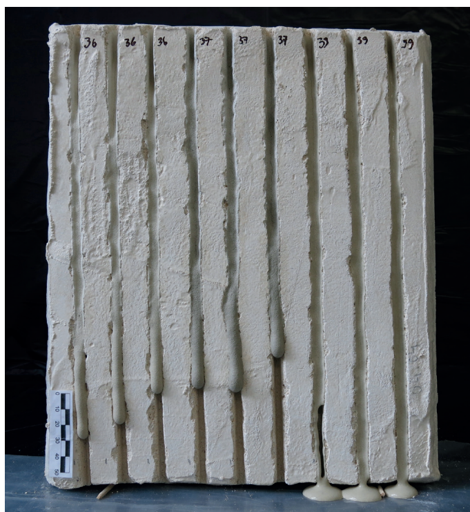
Pic. 1 Plastered panel for the fluidity test. Photo: Varje Öunapuu
