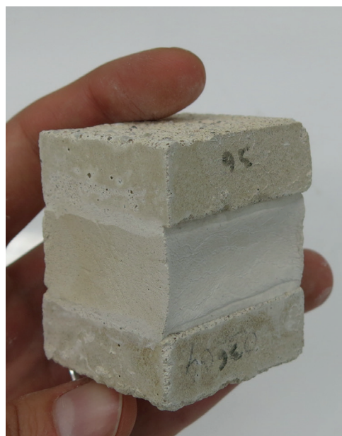
Pic. 6 Prepared test specimen for the adhesion test. Cured injection grout between two pieces of imitation mortar. Photo: Varje Õunapuu
