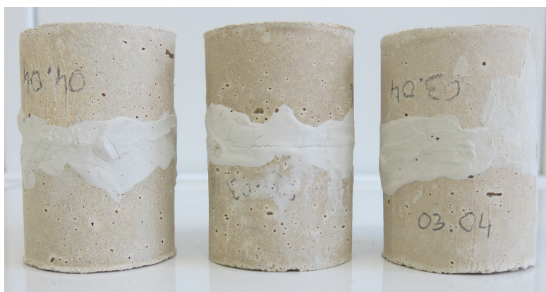
Pic. 2 and 3 Cylinders glued together with the mixture of NHL5 and water. Photos: Varje Õunapuu
